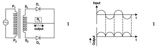
During +ve half cycle diode  $D_1$  is forward biased and diode  $D_2$  is reverse biased. The forward current flows due to  $D_1$ . During –ve half cycle, diode  $D_1$  is reverse biased and diode  $D_2$  is forward biased. The forward current flows due to  $D_2$ . The output waveforms is shown in figure. **1**
