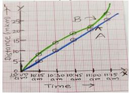
The Position-time graph for object A is a straight line and gives information that motion of object A is uniform, whereas for object B the shape of graph is a curved line and so the motion of object B is non-uniform.
