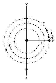
dir<sup>*n*</sup> of  $\stackrel{\rightarrow}{B}$  is along the tangent to mag. field line at that point.
