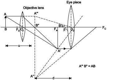
Magnifying power of compound microscope is defined as ratio of angle subtended by final image and object on eye when both are at least distance of distinct vision. 1
