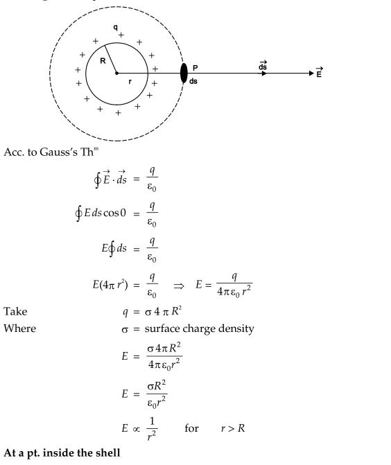
$\oint \vec{E} \cdot \vec{ds} = \frac{q}{\varepsilon_0} \quad \because \quad q = 0 \text{ inside the gaussian surface}$ E = 0
