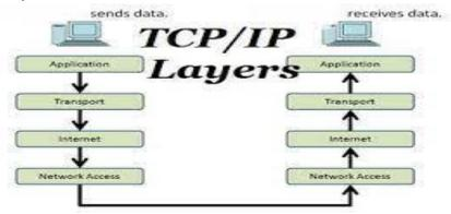
**Application Layer:** An application layer is the topmost layer within the TCP/IP model. When one application layer protocol needs to communicate with another application layer, it forwards its information to the transport layer.
