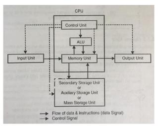
The block diagram of a computer system
